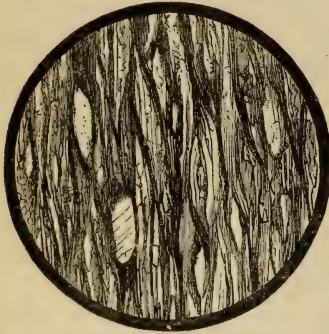
FIG. 72.—SECTION OF COMPRESSED ARGILLACEOUS ROCK IN WHICH CLEAVAGE STRUCTURE HAS BEEN DEVELOPED. MAGNIFIED.
